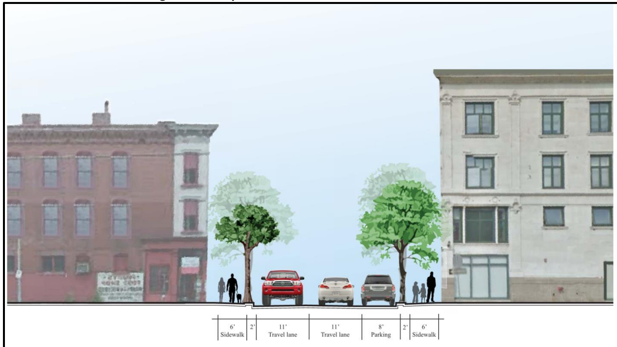
Figure 9 – Proposed Cross-Section on Wallace Avenue
